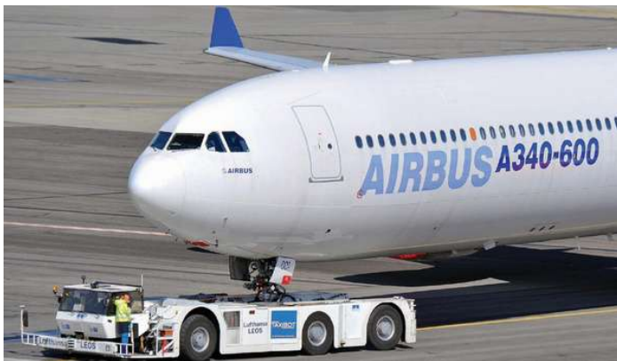
Figure 5: A TaxiBot from IAI operating at the Toulouse Airport with a Airbus A340-600
